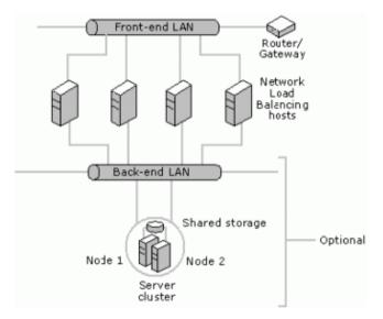
A four-host cluster works as a single virtual server to handle network traffic. Each host runs its own copy of the server with Network Load Balancing distributing the work among the four hosts.
