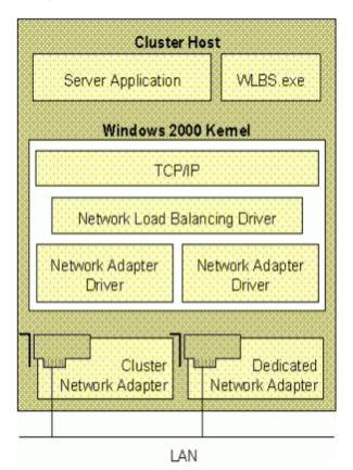
create, delete, append, etc. Could have a backup standby Data node stores file chunks Data nodes may fail arbitrarily, and be added dynamically Scale:  $\times 10$ , 000 Both name node and data node are capable of computation and storage. Network Load Balancing runs as a network driver logically situated beneath higher-level application protocols, such as HTTP and FTP. Figure 2 below shows the implementation of Network Load Balancing as an intermediate driver in the Windows 2000 network stack.
