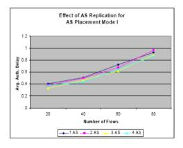
Simulation results showing authentication delay as the number of flows increases from 20-80 flows for 1-4 authentication servers placed using model I. Delay of each set of flows is averaged over 10 simulation runs
