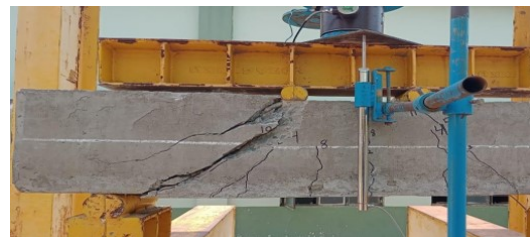
Fig. Specimen tested with spiral stirrups
