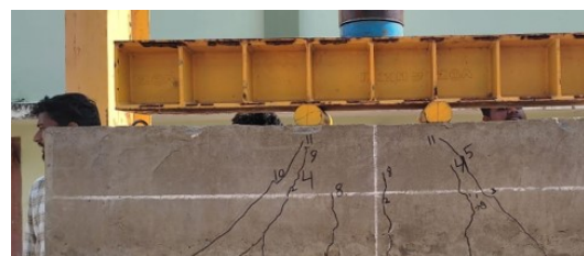
Fig. Specimen tested with vertical stirrups
