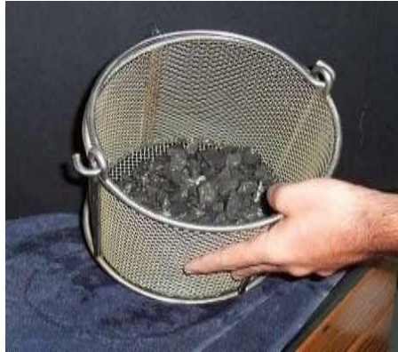
Figure 11: Los Angeles abrasion test apparatus
