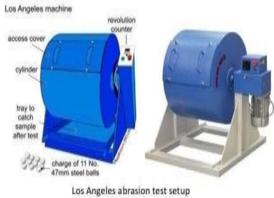
Figure 11: Los Angeles abrasion test apparatus
