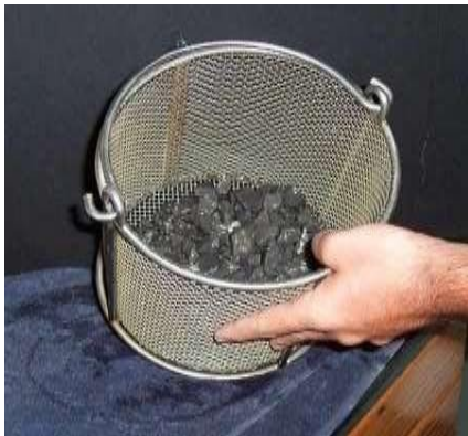
Figure 10: Specific gravity and Water absorption test apparatus
